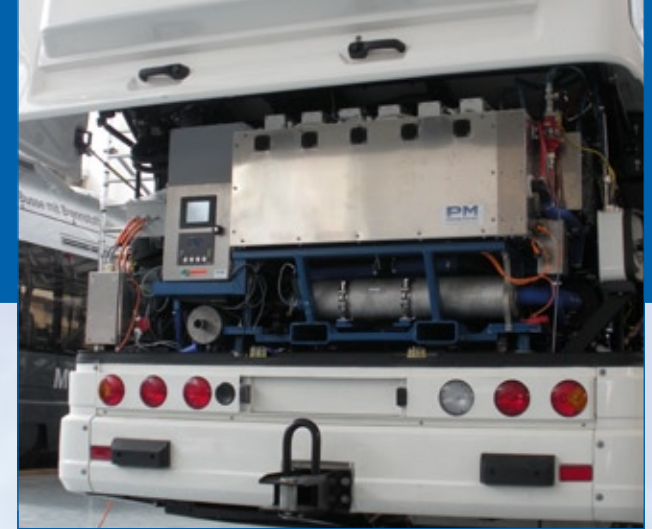
Fuel Cell System integrated into the bus
